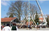
**Photo: BKL\_LTM 1070-4.2.jpg:** A mobile crane from BKL raising a maypole: the LTM 1070-4.2 secures the tree with its mast, extended to approximately 50 metres, and 10.7 tonnes of ballast. (Photo credit: BKL)
